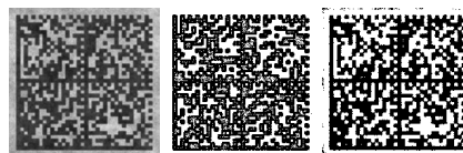
Figure 16. (Case 2) Wetting ink on rough high porosity white paper
