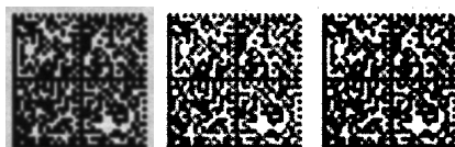
Figure 20. (Case 4) Wetting ink on white, rough, low porosity paper
