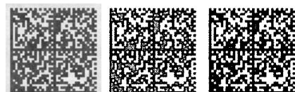
Figure 14. (Case 1) Non-wetting ink on smooth low porosity paper (ideal profile)
