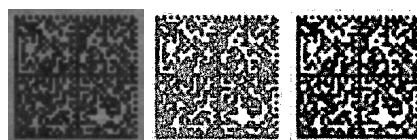
Figure 18. (Case 3) Wetting ink on Dark, Rough high porosity paper
