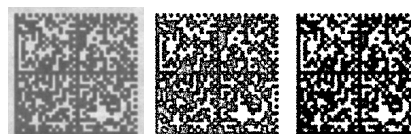
Figure 22. (Case 5) Wetting ink on smooth, low porosity paper
