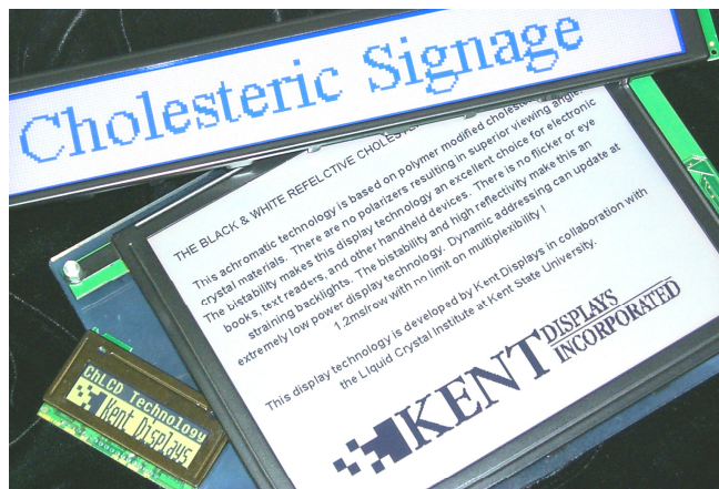
Figure 1. Various ChLCDs in typical office lighting. Shown in the photograph are the wide 12.1" sign type display (blue/white), large 9.4" electronic book type display (black/white), and small 2.3" instrumentation type display (green/black).
