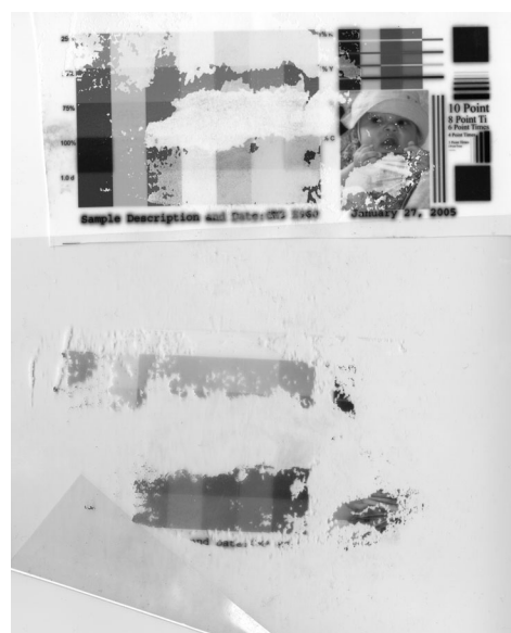
Figure 1. Inkjet material in the presence of Swiffer® was so badly softened that it transferred to the MYLARTM.
