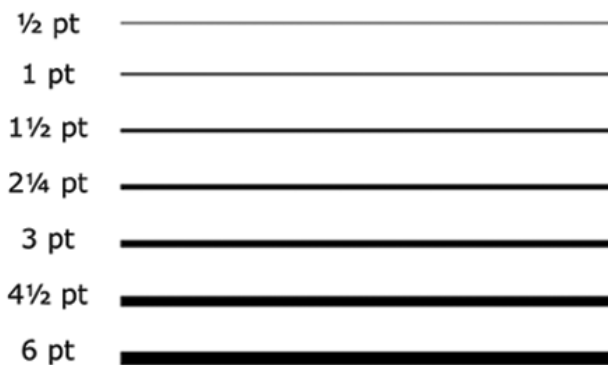
Figure 2. The part of the black & white flat control test printout on microcapsule paper – The test of lines width.
