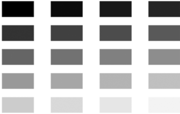
Figure 4. Control test printout of rectangles with various degrees of darkness and its relation to the height of convex rectangles.
