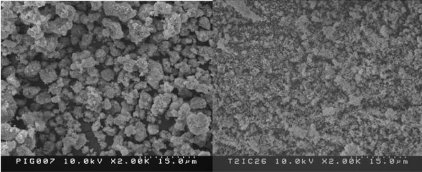
Figure 6. Commercially available precipitated calcium carbonate (left) and its ball-milled calcium carbonate (right)
