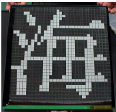
Figure 15. Image sample: the display mode is a passive matrix
