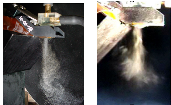
Figure 9. Spray pattern with one shot flash in different electrical power.
