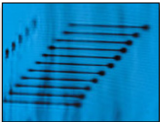
Figure 3. Eleven jets fire simultaneously from one channel
