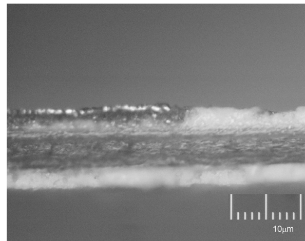
Figure 2. Cross sectional view of PIJ patterned film
