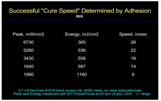
A simple, but dramatic conclusion can be drawn from this data: the adhesion and cure speed of this ink film benefits significantly from high irradiance. At the same time, the total energy required to produce the desired result is *less*.
