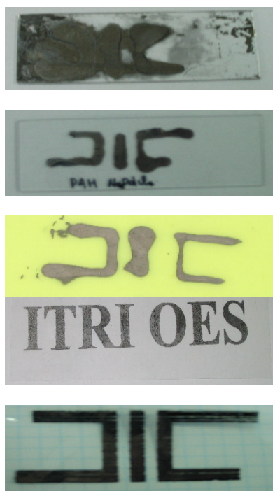
Figure 1(a)-(e). Comparison of ink-jet patterning for different ink solution. All procedures and testing conditions follow Guo et al. report. 10 Three PEMs layer has been on substrate. (a) Drawing outmost PAH pattern on glass substrate, and dipping the glass substrate into catalyst solution, it showed bad selection of Ni, and Ni deposition in backside of glass substrate. (b) Dipping a layer of PAH on glass substrate, and then drawing a catalyst solution pattern on glass substrate. It showed excellent selection of Ni, and no Ni deposition in backside of glass substrate. (c) Dipping a layer of PAH on FR-4 substrate, and then drawing catalyst solution pattern on FR-4 substrate. It showed excellent selection of Ni, and no Ni deposition in backside of FR-4 substrate. (d) Dipping a layer of PAH on PET substrate, and then ink-jet printing catalyst solution on PET substrate. It showed excellent selection of Ni, and no Ni deposition in backside of PET substrate. (e) Dipping a layer of PAH on PET substrate, and then ink-jet printing catalyst solution on PET substrate. It showed excellent selection of Cu, and no Cu deposition in backside of PET substrate.
