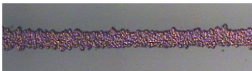
Figure 4. Cu metal line forming by ink-jet catalyst and electroless plating. The average line width is about 92 \mu\text{m} .
