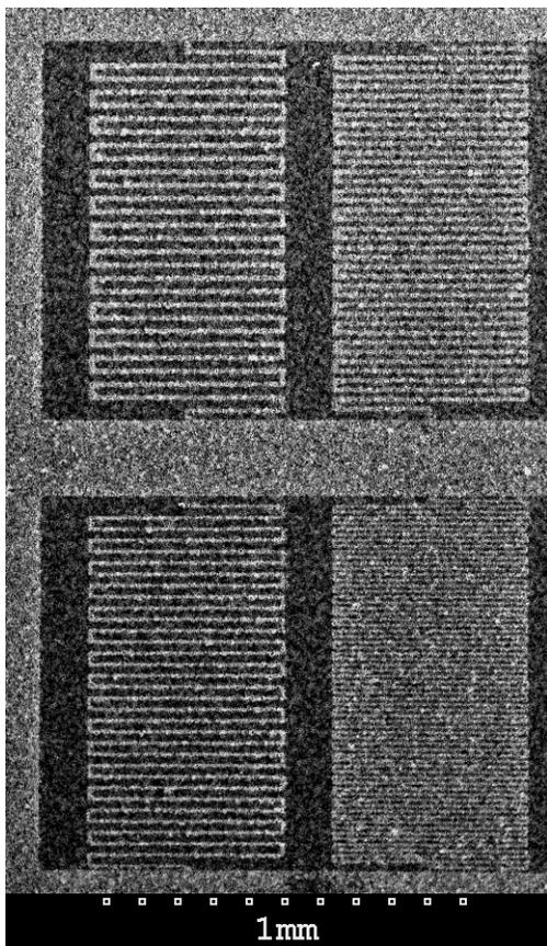
Figure 3. Silver/palladium powder deposited on 10 (top) and 5  $\mu\text{m}$  (bottom) electrode pattern lines and transferred by lamination to a DuPont 951 LTCC particulate tape.
