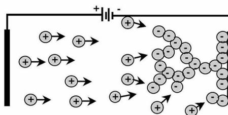
Figure 4. In electrostatic deposition of conductive particles the particles assume the charge of the deposition electrode.
