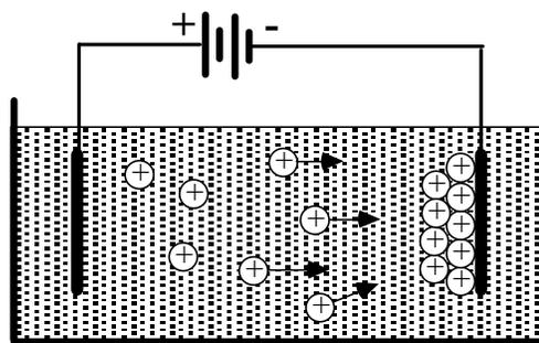
*Figure 1. Positively charged particles will migrate to, and deposit on, a negative electrode surface.*
