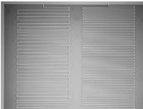
Figure 2. 5  $\mu\text{m}$  wide serpentine lines on deposition pattern.
