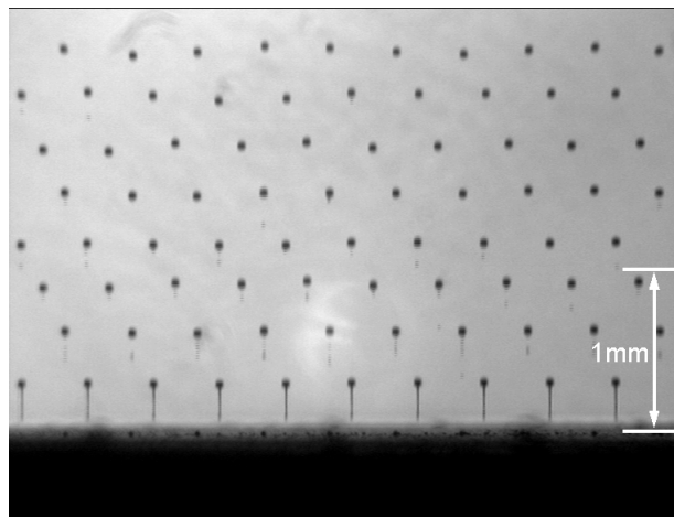
Figure 2. Inkjet drop formation with a well-adapted PEDOT-PSS ink at 6.4 kHz (drop speed = 6 m/s).
