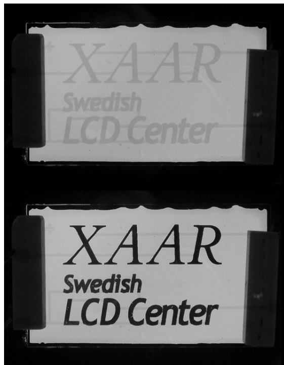
Figure 7. A prototype LCD, with inkjet printed PEDOT-PSS electrodes, in the off and on states.
