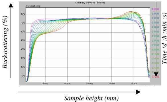
Figure 2. Superposition of scans with time for an unstable sample
