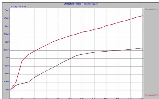
Figure 13. Clarification layer thickness at 30°C (purple) and 40°C (red) as a function of time.
