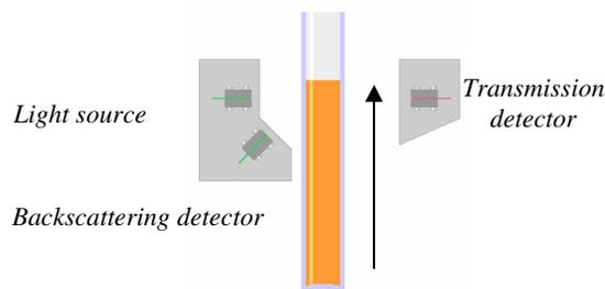
Figure 1. Principle of Turbiscan<sup>®</sup> measurement
