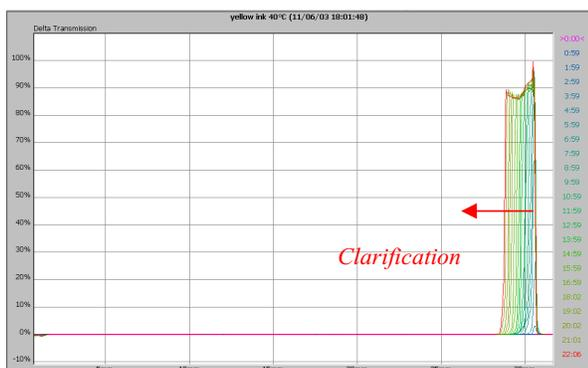
Figure 6. Transmission profile of yellow ink (raw data).
