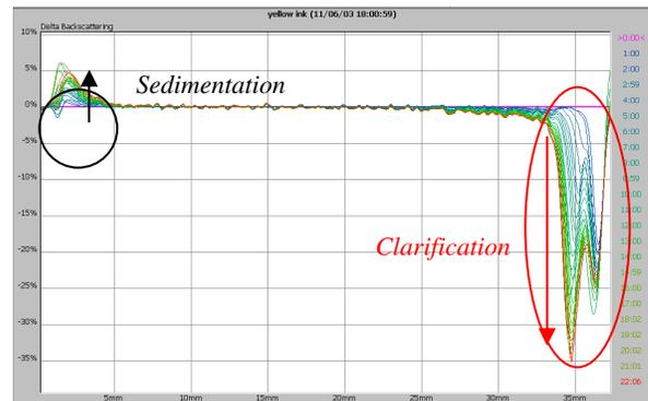
Figure 5. Backscattering profile of yellow ink (reference mode).
