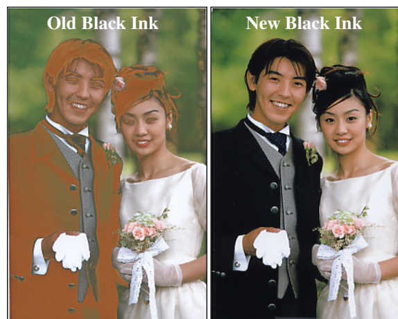
Figure 2. Test samples of Ozone-fastness(after 480ppm·h) of New Black Ink and Old Black with New Color Inks on PGPP
