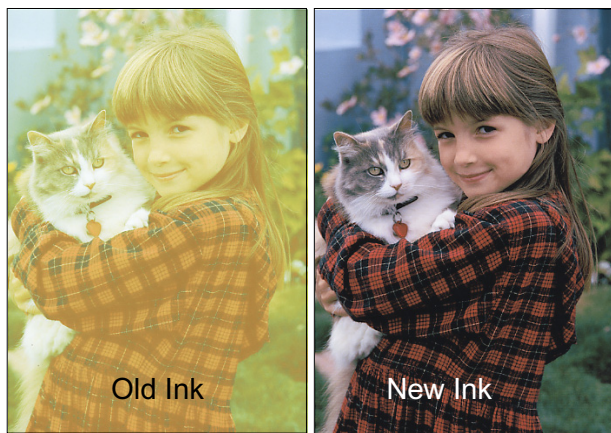
Figure 4. Test samples of Ozone-fastness (after 400ppm·h) of Old Ink and New Ink on PGPP
