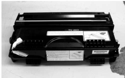
Figure 2. Appearance of the process unit of HL-1240.
