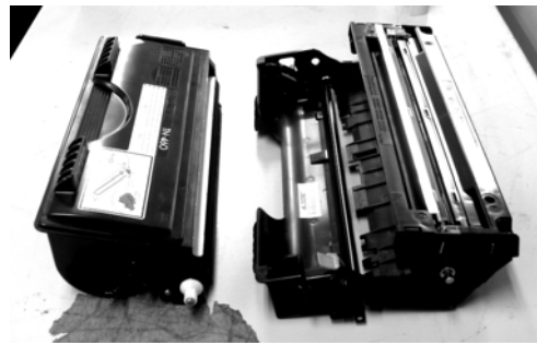
Figure 5. Separating the process unit of HL-1240.
