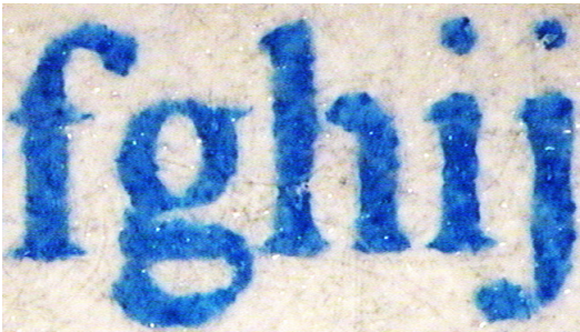
Figure 4. 5 pt characters produced at 1.5m/s print speed using HVT process
