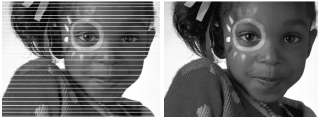
Figure 2. Samples printed with printheads suffering catastrophic damage without correction (left) and after automatic detection and correction (right)
