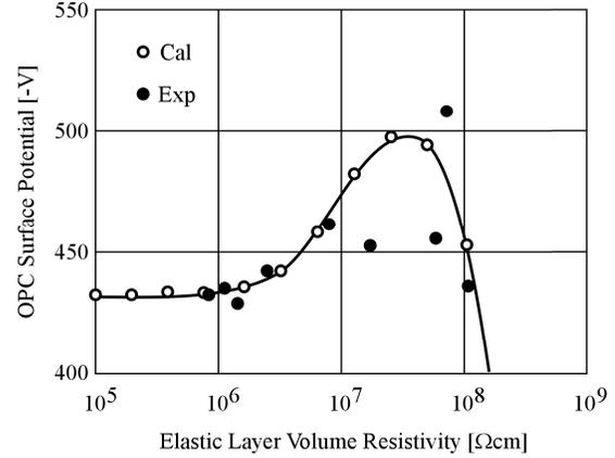
Figure 4. Relationships between OPC Surface Potential and Elastic Layer Volume Resistance. ( $V = -1000$  [V])
