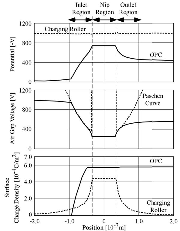
Figure 5. Distribution of Potential, Air Gap Voltage and Surface Charge Density. ( $V = -1000$  [V],  $R_r = 1 \times 10^6$  [ $\Omega$ cm])
