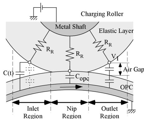
Figure 1. Schematic Diagram of Charging Roller Nip Regions
