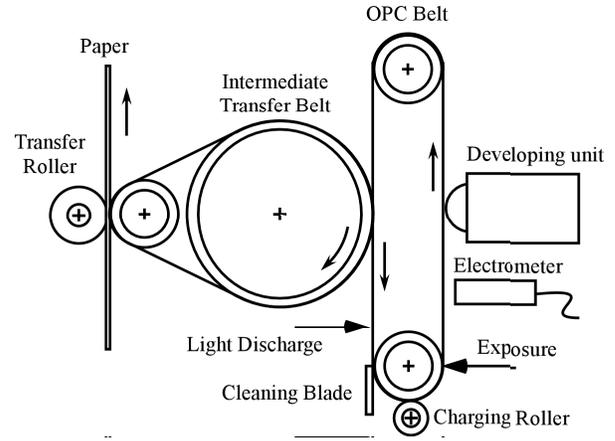
Figure 2. Schematic Diagram of the Experimental Apparatus
