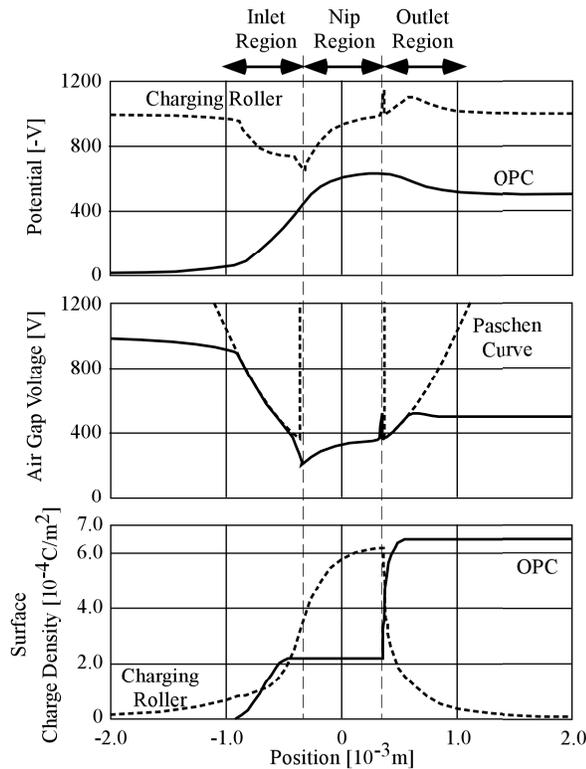
Figure 6. Distribution of Potential, Air Gap Voltage and Surface Charge Density. ( $V=-1000[V]$ ,  $R_r=5 \times 10^7 [\Omega \text{ cm}]$ )
