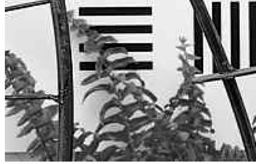
Figure 4. JPEG Decoded Image (a part of SCID N5A) PSNR: 27.086 [dB], Bit Rate: 1.56bits/pixel
