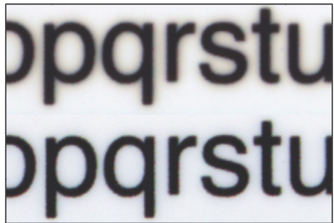
Figure 8. Text printed on system having Black/white color pair line Bleed Rating = 3.0. Top row is "after" humidity exposure.
