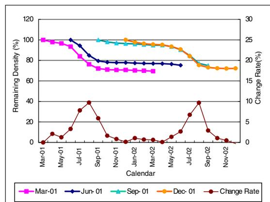
Figure 1. Fading behavior on PGPP of Cyan on bare samples hung indoors in Japan. (Four samples, evaluated from Mar/01 to Dec/02)
