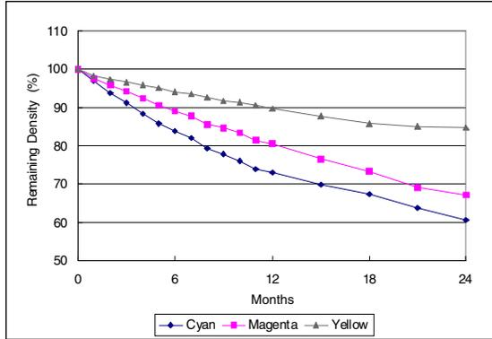
Figure 3. Fading behavior of pure color bare samples on PGPP indoors in Japan. (Average of 40 samples)
