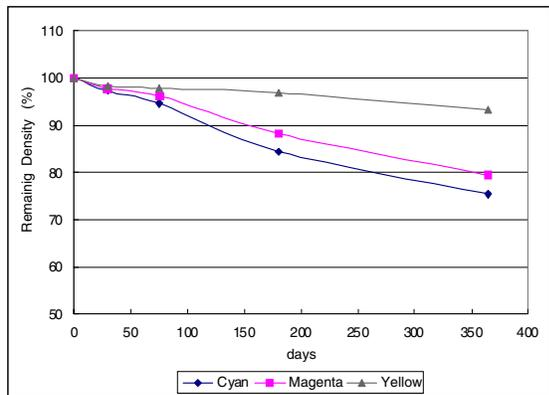
Figure 4. Fading behavior on PGPP of pure color bare samples hung indoors around the world.
