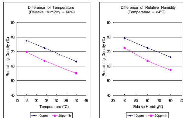
Figure 8. The effect of temperature and relative humidity on fading behavior on PGPP during ozone exposure.
