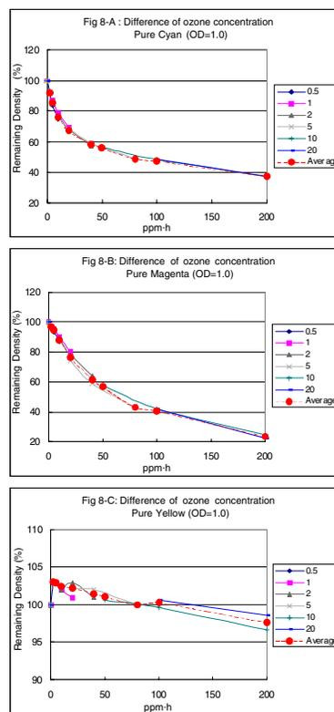
Figure 9. The impact of ozone concentration on fading behavior on PGPP during ozone exposure.
