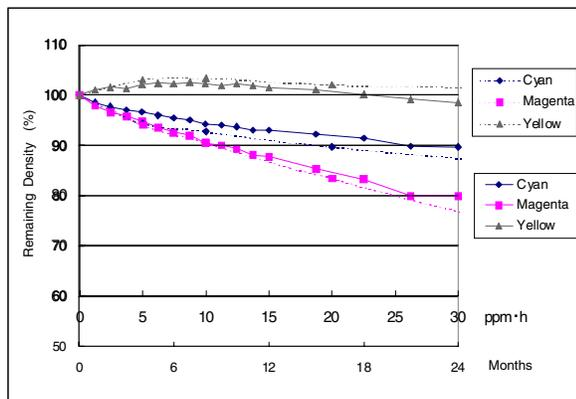
Figure 7. The correlation between bare samples hung indoors in Japan and ozone exposure on MPH. (Solid Line: Indoors, Dotted Line: Ozone)
