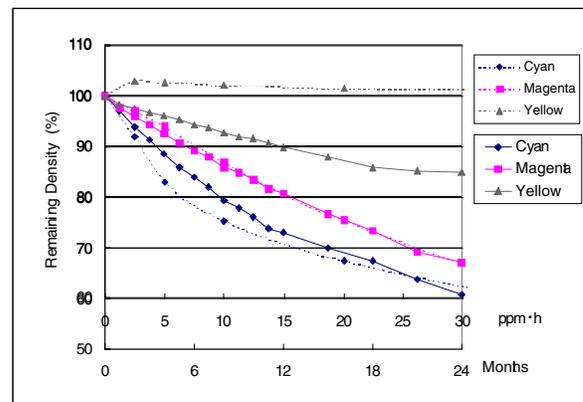
Figure 6. The correlation between the bare samples hung indoors in Japan and ozone exposure on PGPP. (Solid Line: Indoors, Dotted Line: Ozone)
