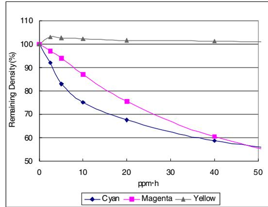
Figure 5. Fading behavior of pure color on PGPP under ozone exposure.
