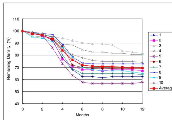
Figure 2. Fading behavior on PGPP of Cyan on bare samples hung indoors in Japan. (Evaluation period: Mar/01-Mar/02)
