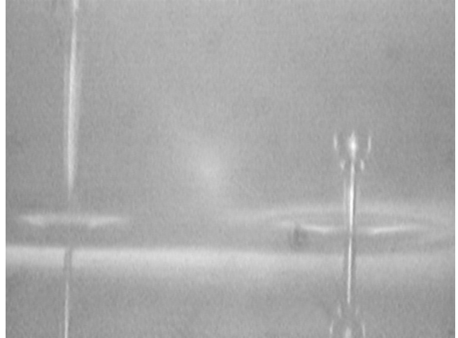
Figure 3. Only the left channel is fired but also the right channel ejects a droplet because of the crosstalk effect.
