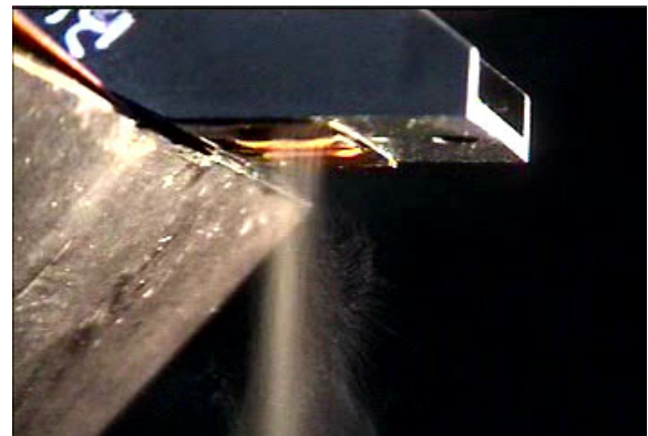
Figure 8. Fuel ejection of the thermal fuel injector
