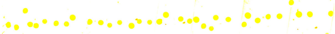
Figure 9. The photographical image of dots printed-out actually by type NZ-B2 with 36 nozzles (3 dots lost).
