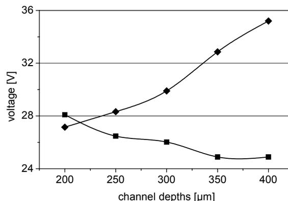
Figure 5. The voltage amplitude required to reach  $6\ \text{m/s}$  drop velocity versus the channel depth  $D_C$  or  $D_B$  for the upper (■) and lower (◆) channels
