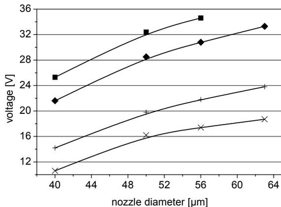
Figure 8. The driving voltages required to obtain ink drop velocities of 6 m/s plotted against the nozzle diameter. Chevron type offset-channel printheads (× upper channel, + lower channel) require strongly reduced driving voltages as compared to their monolithic counterparts (◆ upper channel, ■ lower channel).
