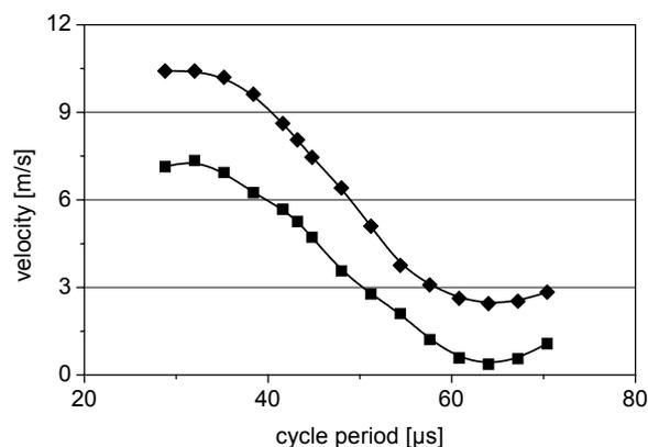
Figure 3. Response curves of an offset-channel printhead with  $D_C$  (■) =  $D_B$  (◆) =  $300\mu\text{m}$
