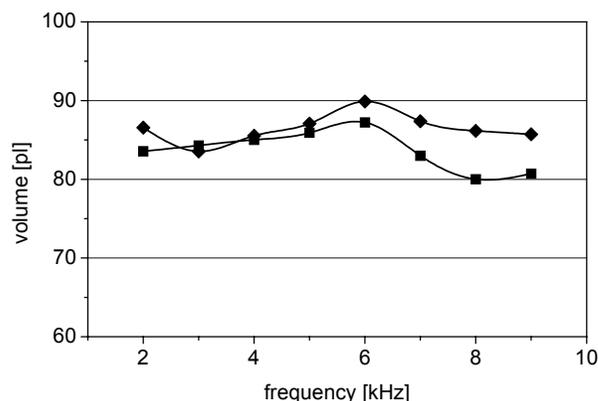
Figure 6. No starvation was observed up to  $9\ \text{kHz}$  print frequency for both of the offset-channels with large channel depth,  $D_C = D_B = 400\ \mu\text{m}$ , i.e. the upper (■) and lower (◆) channels, respectively
