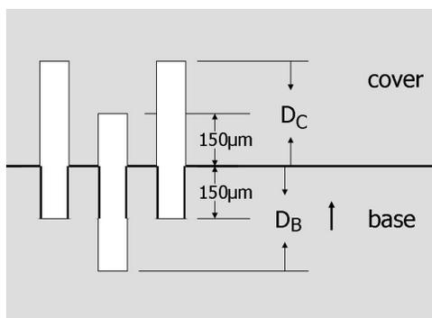
Figure 2. Cross section of an 'offset-channel' actuator.  $D_C$  and  $D_B$  represent the channel depth in the cover and the base, respectively.
