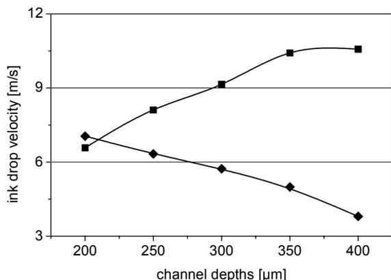
Figure 4. The ink drop velocity as a function of channel depth  $D_C$  or  $D_B$  for the upper (■) and lower (◆) channels
