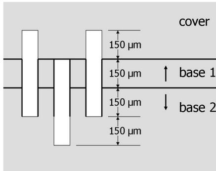
Figure 7. The Chevron version of the offset-channel actuator
