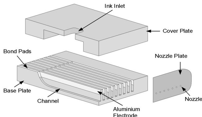
Figure 1. Scheme of an Xaar-type end-shooter printhead
