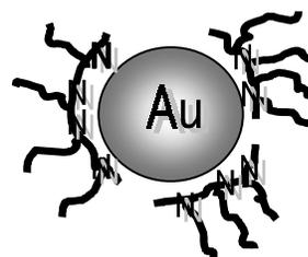
Figure 1. Schematic Illustration of gold nano-particle stabilized by comb-shaped block copolymer
