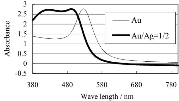
Figure 9. Plasmon light absorption spectra of gold-core / silver-shell nano-particle suspension.
