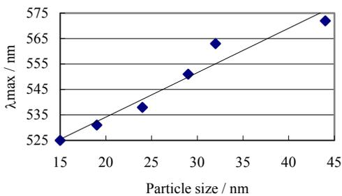
Figure 8. Relation between particle size of gold and wavelength at absorption maximum ( $\lambda_{max}$ )
