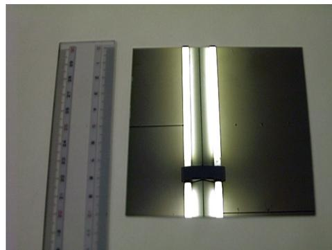
Figure 10. A thin film with metal like appearance using silver nano-particle paste
