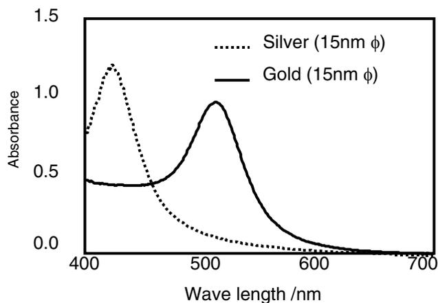
Figure 6. Light absorption spectra for suspensions of silver and gold nano-particles.
