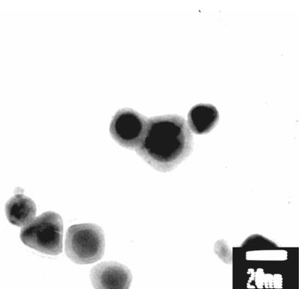
Figure 4. TEM photograph of gold-core / silver-shell alloy nano-particle (Au/Ag=1/2 by weight)
