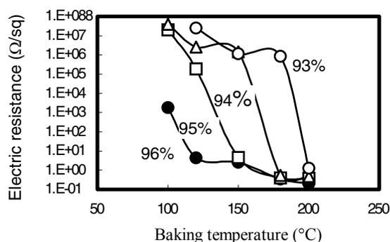
Figure 11. Surface electro-resistance of films containing silver nano-particle as functions of baking temperature at different silver contents
