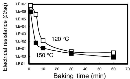
Figure 12. Electro-conductivity of films containing 96% of silver nano-particles as functions of baking time
