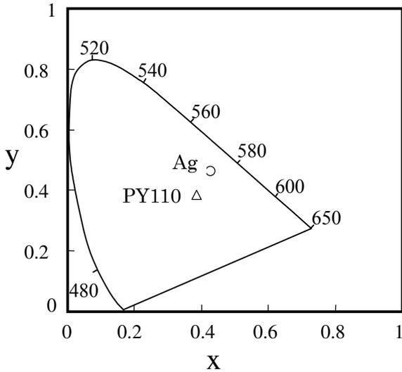
Figure 7. Comparison of color saturation between silver nano-particle and Pigment Yellow 110
