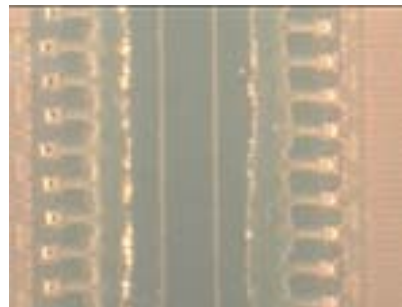
Figure 1. Ink Channels and Nozzle, Thermal ink Jet Head
