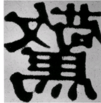
Figure 4. Developed toner image on the photoreceptor with RD rotation.
