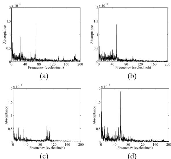
Figure 5. Spectra of projected absorptance for (a) LJ 1000, (b) LJ 4050, (c) ML-1450, and (d) LJ 1200
