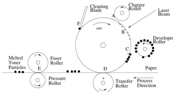
Figure 3. Electrophotographic process: cross sectional view of typical laser printer (A) Charging (B) exposure (C) development (D) transferring (E) Fusing and (F) cleaning.
