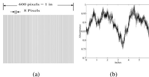
Figure 4. (a) Test pattern for 12.5% fill gray level patch and (b) 1-D horizontal projection of the printed and scanned test pattern. Each row of the test pattern consists of a repeating pattern of a one followed by seven zeros. The test pattern was scanned at 600 dpi.
