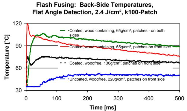
Figure 3. Time dependence of backside paper temperature after flash fusing for different conditions
