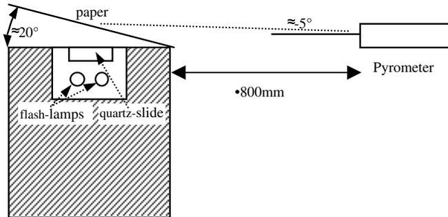
Figure 2. Experimental setups to measure paper backside temperature at flash fusing
