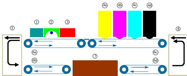
Figure 5. Breadboard for duplex color printing using UV-curing toner
