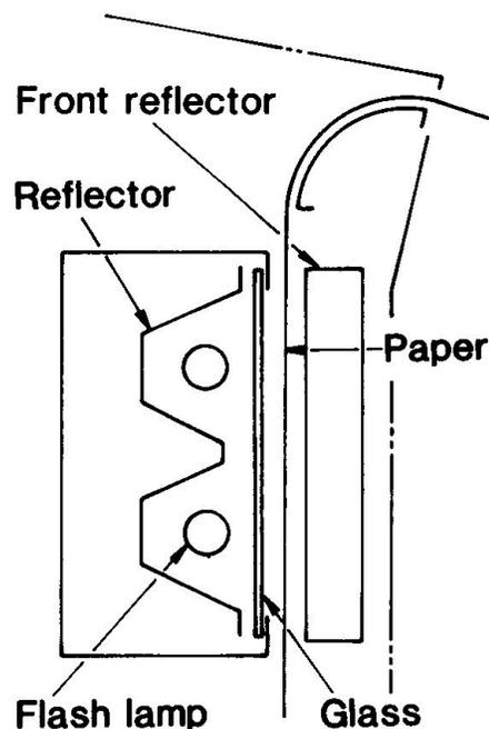
Figure 1. Structure of color flash fuser<sup>6</sup>
