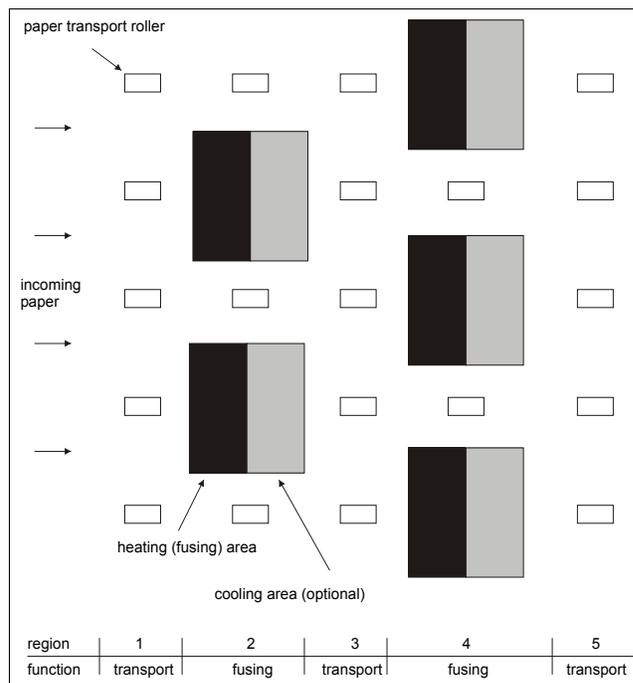
Figure 4. Schematic view of the staggered transport path with action areas of heaters and coolers
