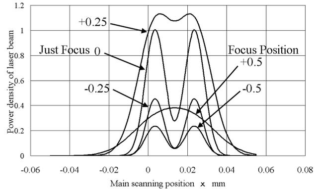
Figure 3. Laser beam profiles according to focus positions
