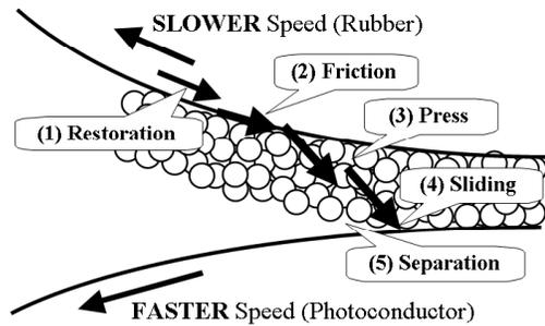
Figure 7. The estimated mechanism of the shearing transfer process
