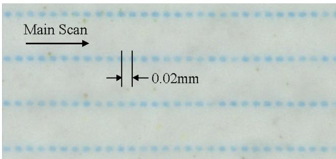
Figure 6. The dots formed on a paper
