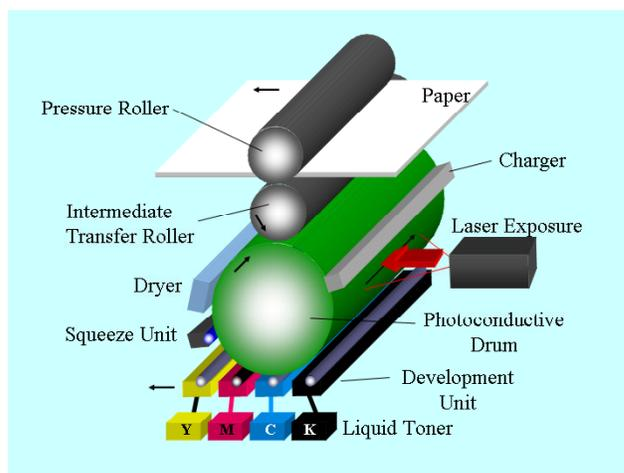
Figure 1. Configuration of the liquid electrophotography system
