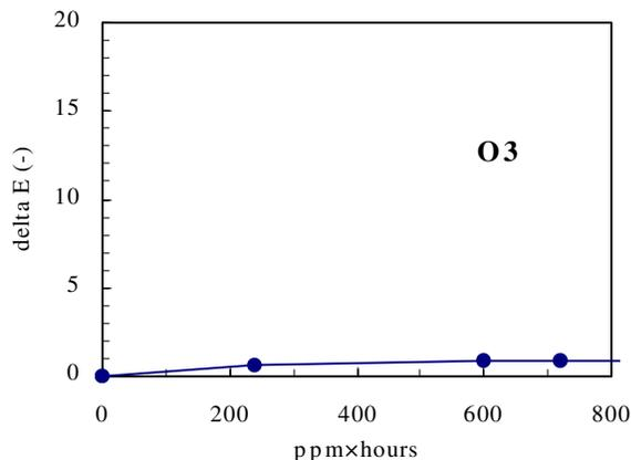
Figure 2(a). Test results of the O<sub>3</sub> at 24°C×60%RH
