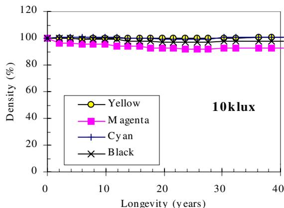
Figure 1(b). The Lightfastness of prints using PLPP. The test was maintained at 10 Klux×24°C×55%RH
