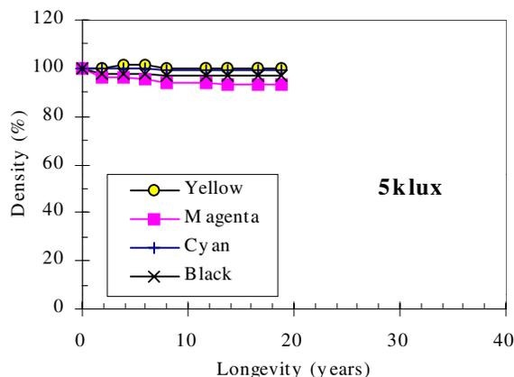
Figure 1(c). The Lightfastness of prints using PLPP. The test was maintained at 5 Klux×24°C×55%RH.
