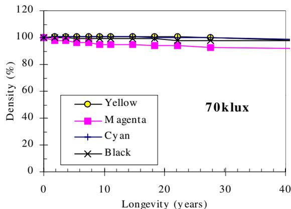
Figure 1(a). The Lightfastness of prints using PLPP. The test was maintained at 70 Klux×24°C×55%RH.
