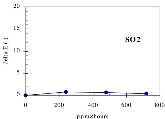
Figure 2(b). Test results of the SO<sub>2</sub> at 24°C×60%RH
