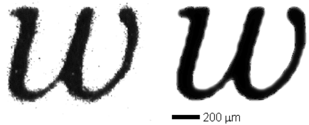
Figure 16. Grayscales for 1200 dpi: scanned 4-point "w" (left) vs. predicted "w" (right)
