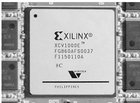
Figure 1. Picture of the hardware component that does color separation and error diffusion
