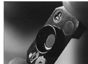
Figure 12. Disposable diagnostic test that contains up to 100 tests printed using ink-jet technology.
