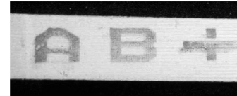
Figure 10. Four antibody test printed using ink-jet technology.
