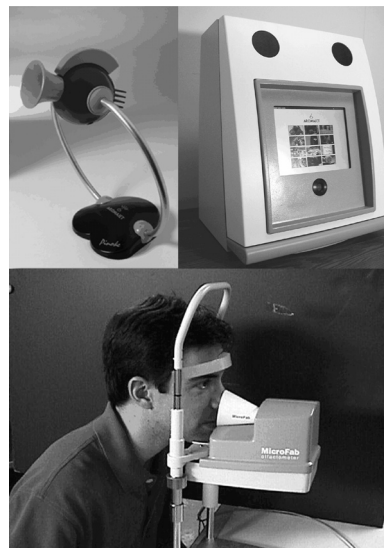
Figure 6. Implementations of Aroma Jet™ technology: top left, 8 aroma desktop computer peripheral; top right, 16 aroma kiosk; bottom, 2 aroma diagnostic instrument.
