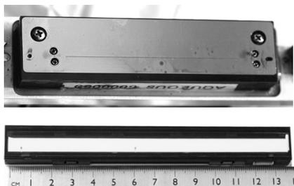
Figure 6. The linear array and Spectra head
