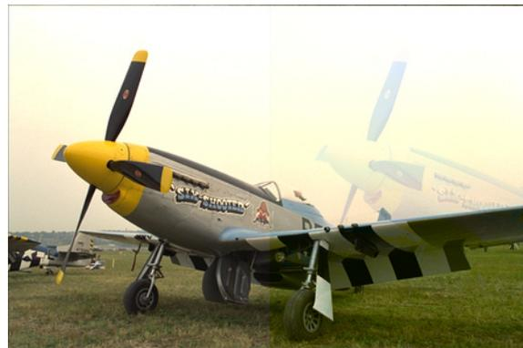
Figure 16: Ghosting simulation image. The front part of the airplane is dimly repeated on the light tone area.
