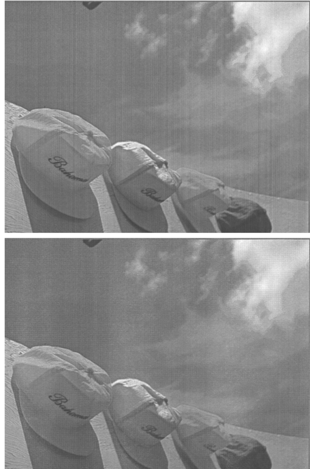
Figure 8. Actual images printed from the uncompensated (top) and compensated (bottom) systems. The compensated system implemented the proposed spatial-based TDOF repetitive controller.
