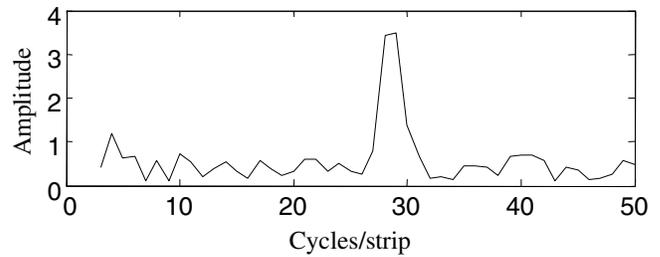
Figure 6. Fourier transform of strip profile
