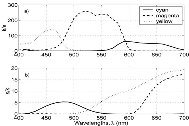
Figure 2. Spectral variation for the relative strength of the absorption and the scattering.
