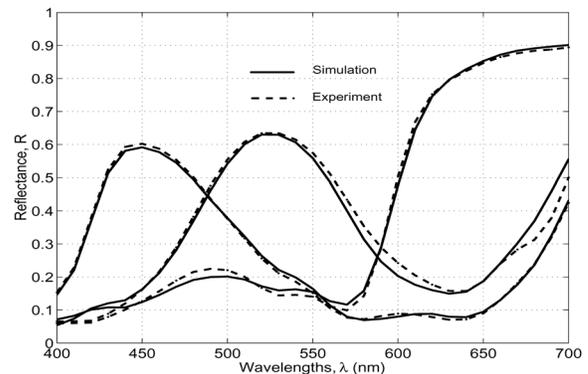
Figure 6. Simulated and measured spectral reflectance values for samples in secondary colors. The samples were printed with program specified ink level 1.
