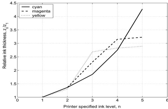
Figure 4. Actual ink volumes  $\alpha = z_n/z_1$  vs. printer driving program specified ink volumes ( $n=1-5$  for ink level 1-5). The actual ink volume for the program specified ink level 1 ( $z_1$ ) has been set as unit for each color.
