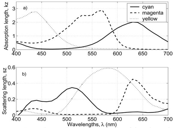
Figure 1. Scattering- and absorption-lengths of the primary inks obtained by fitting into the measured spectral reflectance values of samples printed on ink-jet films with (printer driving) program specified ink level 3.
