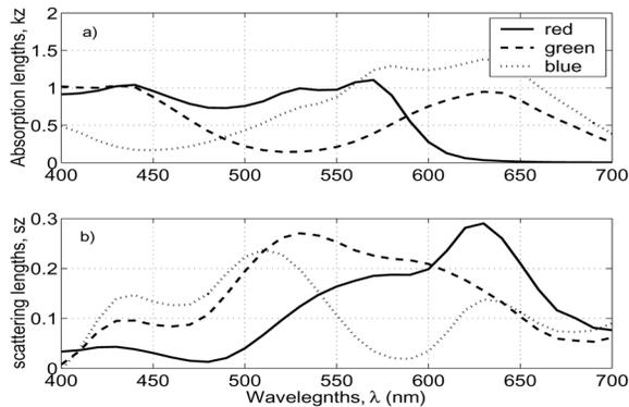
Figure 5. Scattering- and absorption-lengths of the secondary colors obtained by applying the assumption of additivity.
