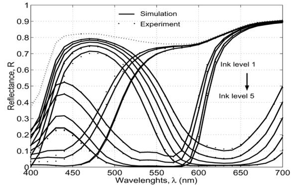
Figure 3. Simulated and measured spectral reflectance values for samples printed with different (printer driving) program specified ink levels. The dot line is the spectral reflectance values of the bare film.
