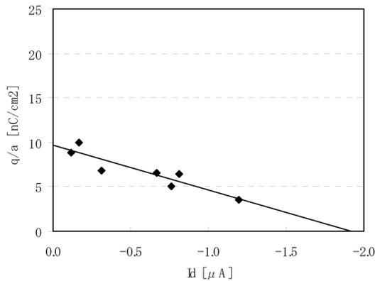
Figure 8. Relationship between  $q/a$  and development roller current ( $I_d$ )
