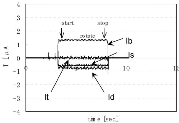
Figure 5. Currents through each part grounded for roller #1.
