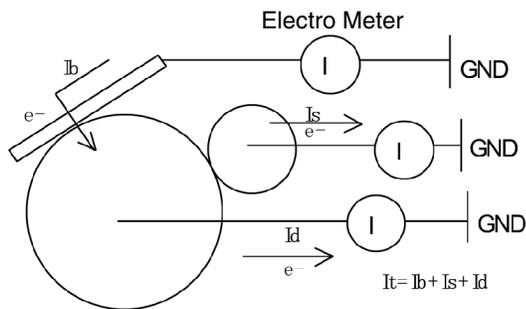
Figure 2. Scheme of current measurements (arrow indicates electron flow).
