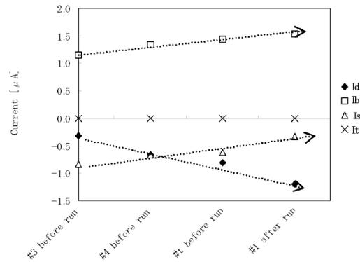
Figure 7. Comparison of currents for rollers #1, #2 (before running test) and roller #1 (after running test).
