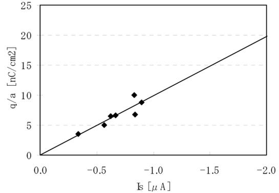
Figure 10. Relationship between  $q/m$  supply current ( $I_s$ ).
