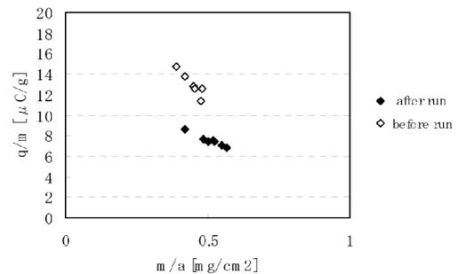
Figure 3.  $q/m$  before and after running for roller #1, grounded.
