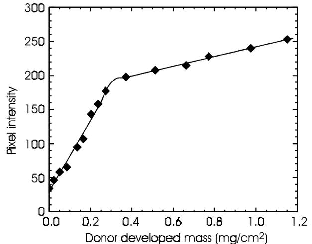
Figure 3. Camera mass calibration
