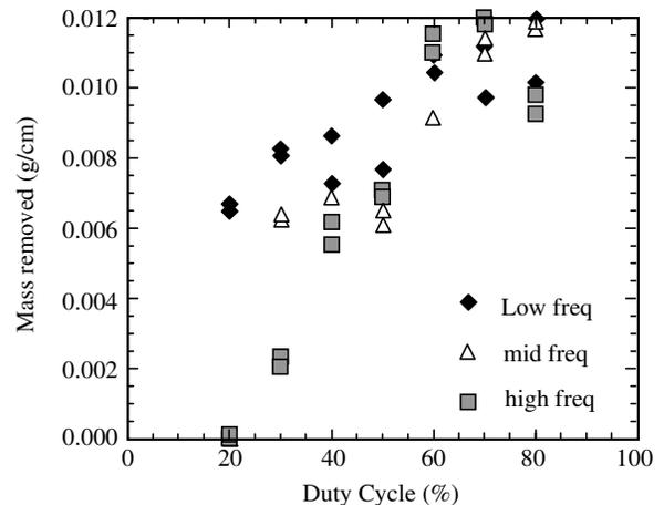
Figure 6. Duty cycle dependence of toner extraction
