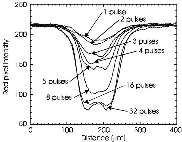
Figure 4. Extracted toner profiles
