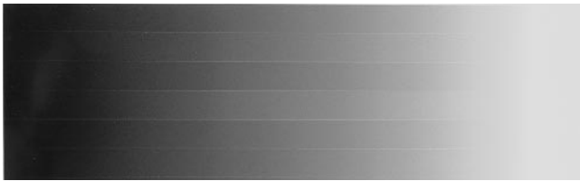
Figure 3 Photograph of real print with color bands due to forced alignment errors
