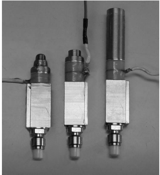
Figure 2. The Jemtex Family of Multi-Deflection Continuous Ink Jet Print Heads
