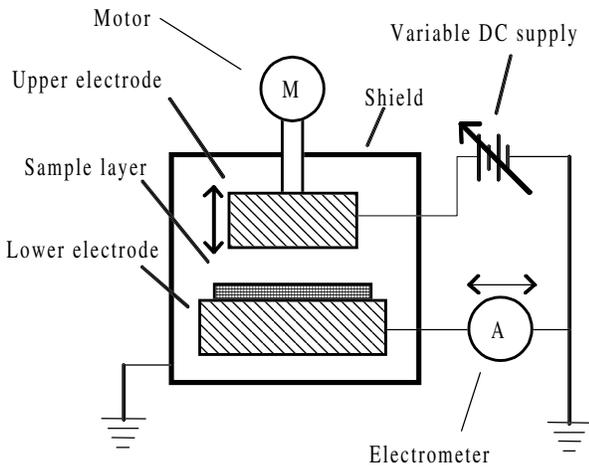
Figure 1. Schematic drawing of an apparatus for contact potential difference measurement.
