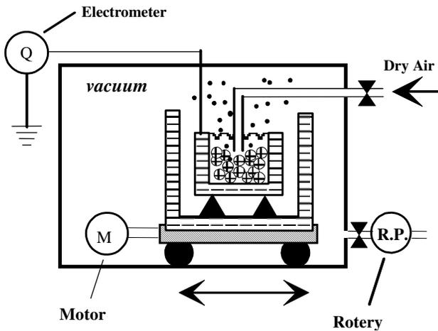
Figure 2. Schematic drawing of an apparatus for measurements of tribocharge between a polymer powder and metal beads.
