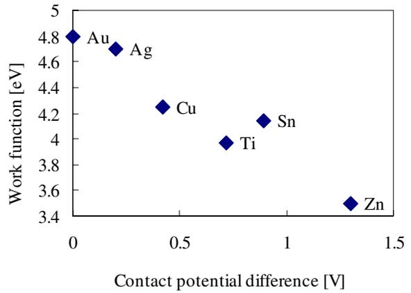
Figure 8. Relationship between work functions and contact potential differences of metal beads after polishing.
