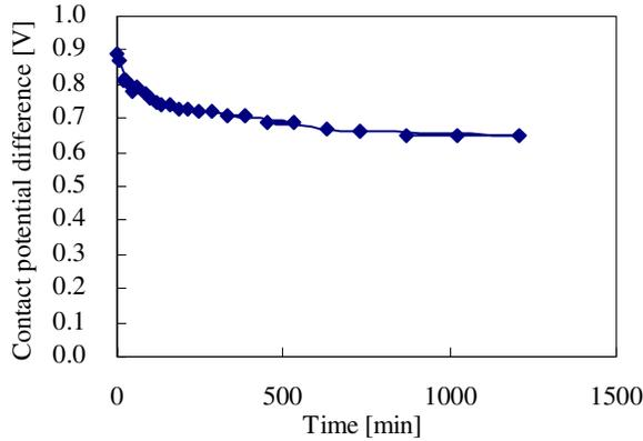
Figure 6. The influence of surface oxide of Ti on its contact potential difference with time after polishing with sandpaper.
