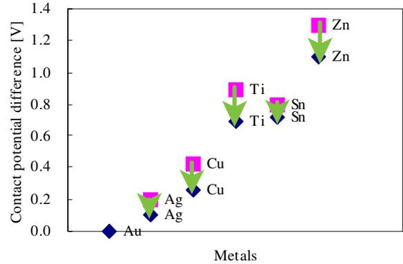
Figure 7. The influence of surface oxide of several metals on contact potential difference with time after polishing for all metal beads used in this study.
