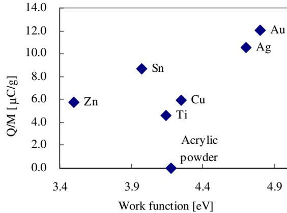
Figure 10. Relationship between  $Q/M$  of acrylic powder and work functions of metal beads after polishing.
