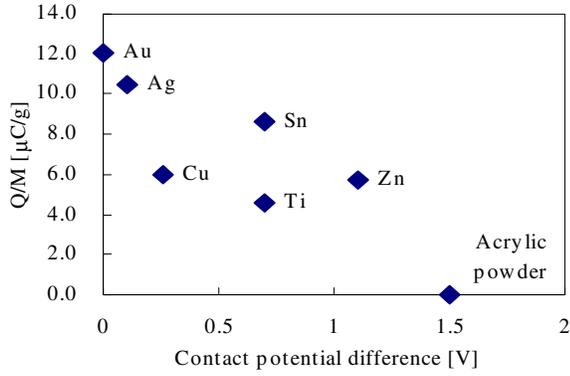
Figure 4. Relationship between  $Q/M$  of acrylic powder and contact potential differences of metal beads.
