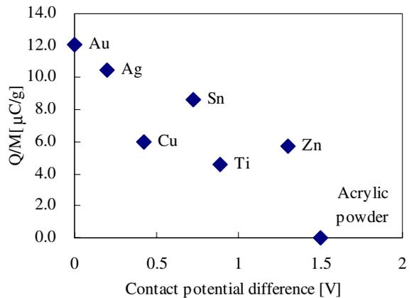
Figure 9. Relationship between  $Q/M$  of acrylic powder and contact potential difference of metal beads after polishing.
