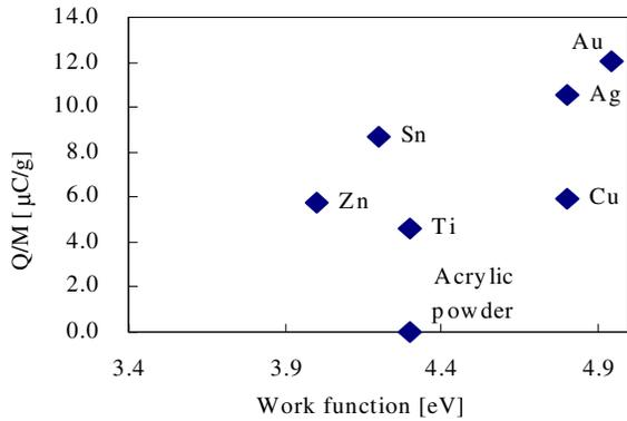
Figure 5. Relationship between  $Q/M$  of acrylic powder and work functions of metal beads.
