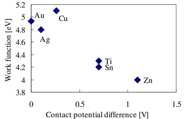
Figure 3. The work functions against contact potential difference to gold.
