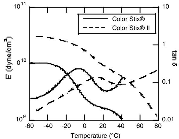
Figure 1. Dynamic Mechanical Analysis Profiles of Color Stix® and Color Stix® II Solid Inks
