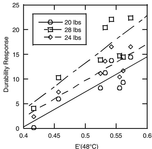
Figure 2. Durability Response versus Storage Modulus(48°C) for Various Media Weights
