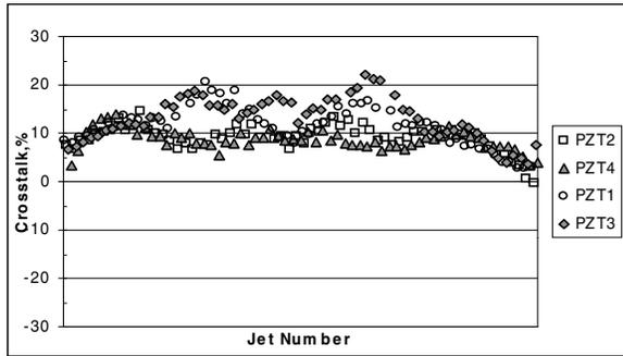
Figure 3. Crosstalk of CCP printhead, measured at 7 kHz, percent deviation from initial jet velocity
