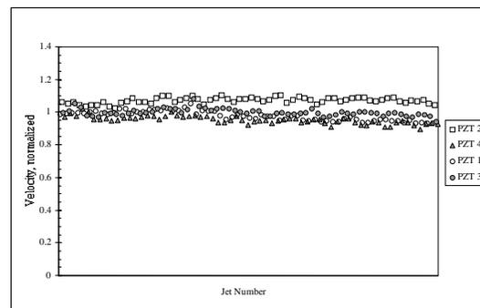
Figure 2. Velocity plot of Galaxy printhead, 8 kHz operating frequency, normalized to head average velocity
