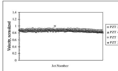
Figure 1. Velocity plot of CCP printhead, 7 kHz operating frequency, normalized by head average velocity of Galaxy printhead.
