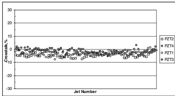
Figure 4. Crosstalk of Galaxy printhead, measured at 8 kHz, percent deviation from initial jet velocity
