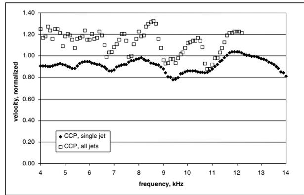
Figure 5. Frequency response with crosstalk of CCP printhead.
