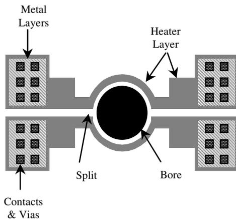
Figure 2. Top view illustration of a single nozzle
