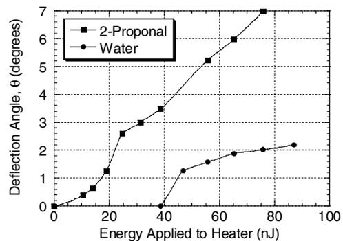
Figure 3. Plot of deflection angle versus energy applied to the heater segment
