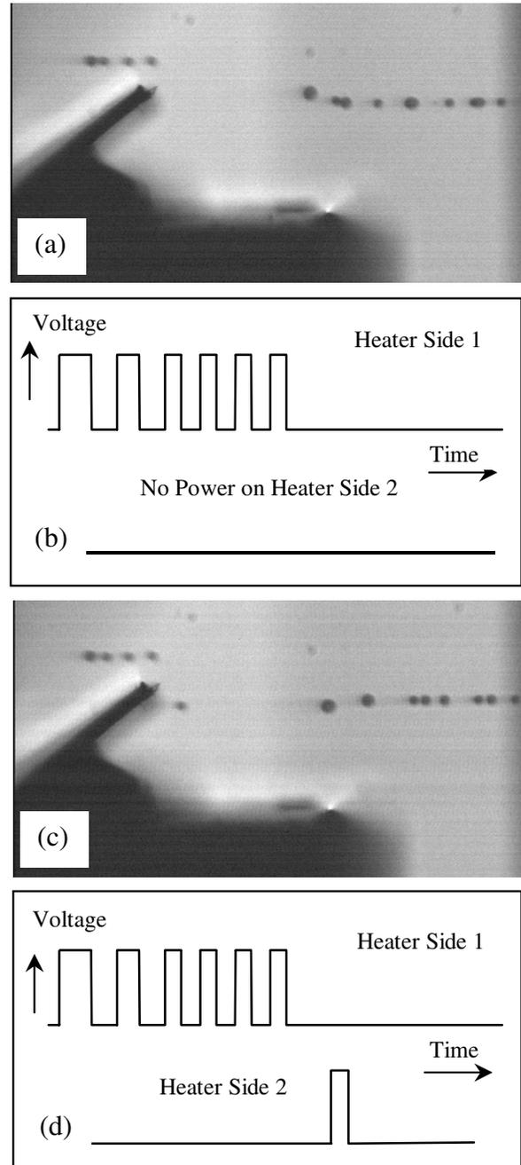
Figure 4. (a) Five-drop burst traveling from right to left with only first heater side powered. (b) Waveform used to create drop bursts  $t$  seen in (a). (c) Five-drop burst using both heater sides. (d) Waveform used to create drop burst seen in (c).
