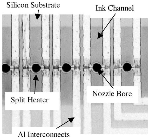
Figure 5. Top view of multi-nozzle printhead
