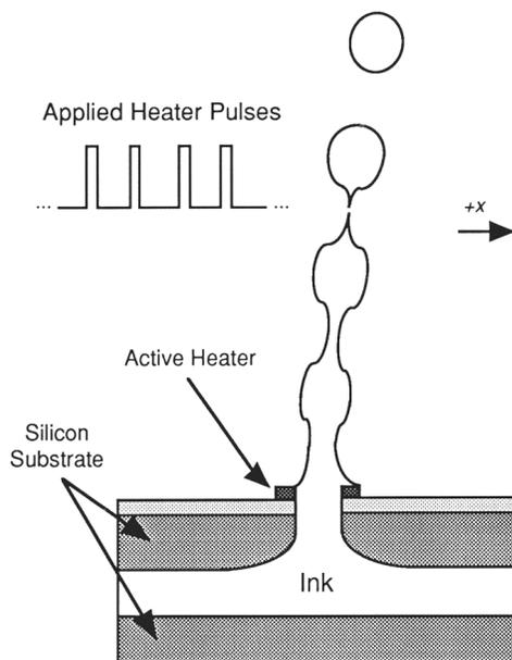
Figure 1. Schematic cross-sectional view of a nozzle
