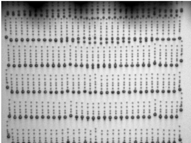
Figure 6. Experimental image of 600 NPI printhead showing 64 columns of drop bursts
