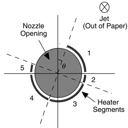
Figure 7. Top view of a nozzle having multiple heater segments used to steer drops
