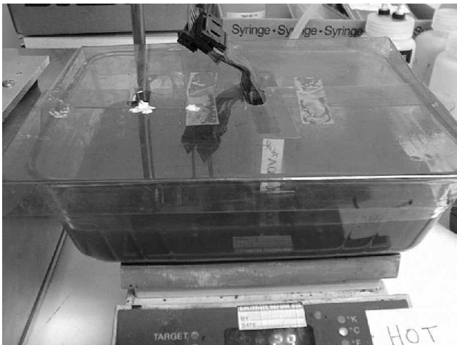
Figure 7. Laboratory setup for immersion testing.
